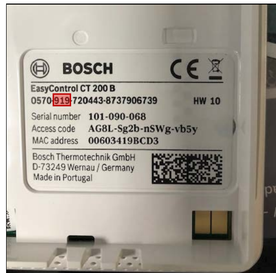
Fig. 2) FD code shown on back of Easy Control unit
